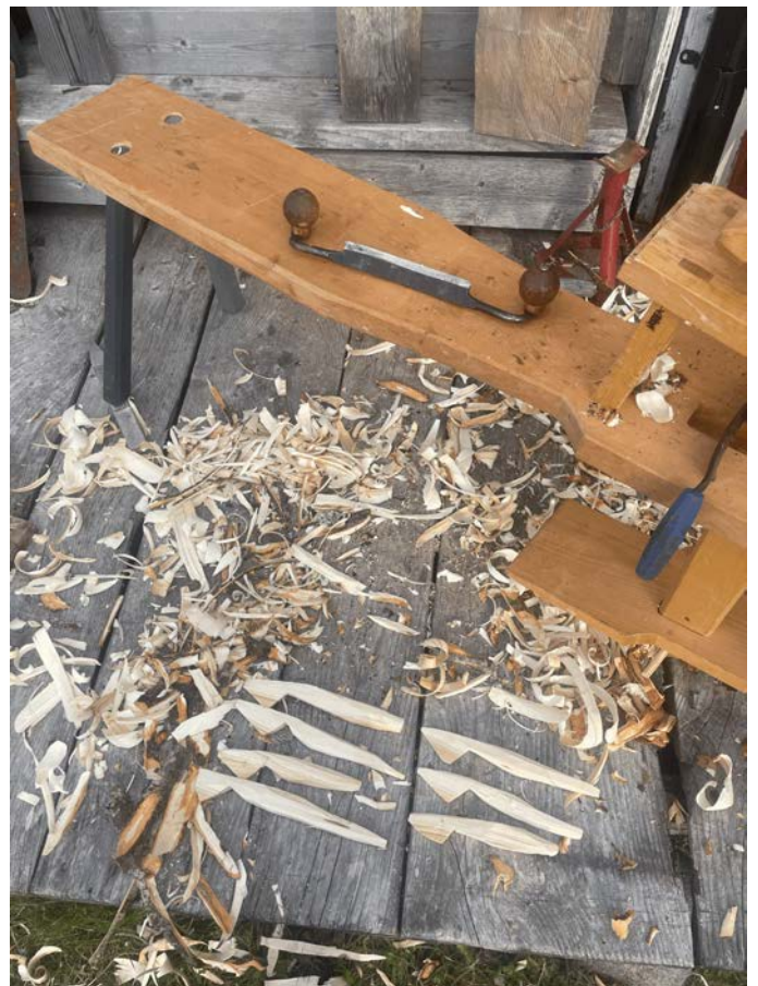
For making rough blanks of butter knives, we used green wood (= fresh and still moist wood) that was shaped with an axe, shaving horse and a drawknife.
