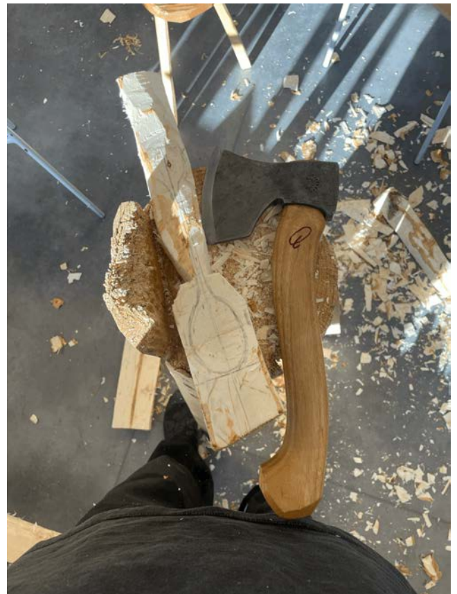
Usually butter knives and spoons were made from split greenwood with an axe, a draw knife, a knife and a spoon knife. No sanding paper was ever used when it came to slöjd.
