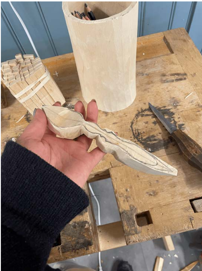
Usually butter knives and spoons were made from split greenwood with an axe, a draw knife, a knife and a spoon knife. No sanding paper was ever used when it came to slöjd.
